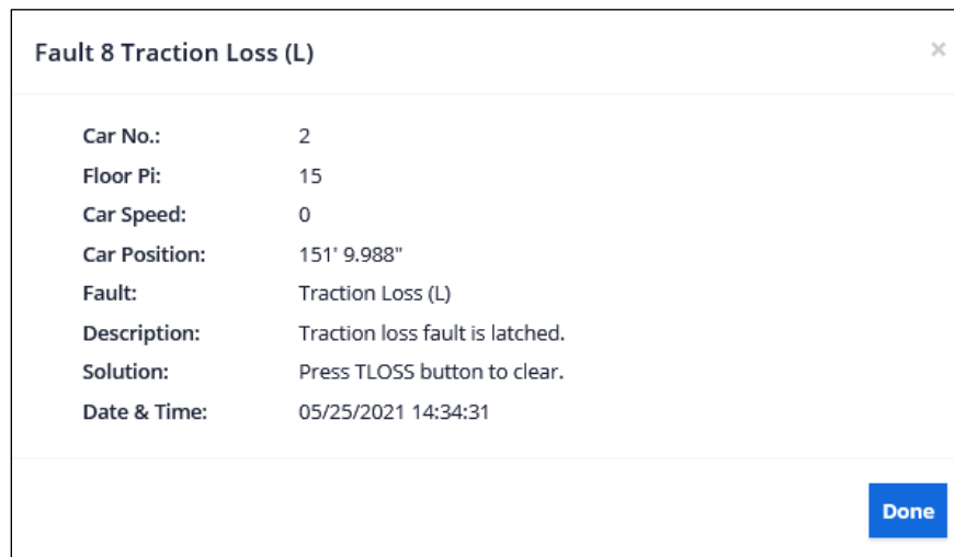
Figure 26: Fault and Traction Loss Pop-up
